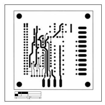
Figure 4. MAX1202 EV Kit PC Board Layout—Solder Side
