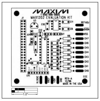
Figure 2. MAX1202 EV Kit Component Placement Guide— Top Silkscreen
