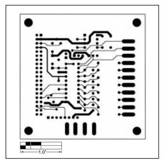
Figure 3. MAX1202 EV Kit PC Board Layout—Component Side
