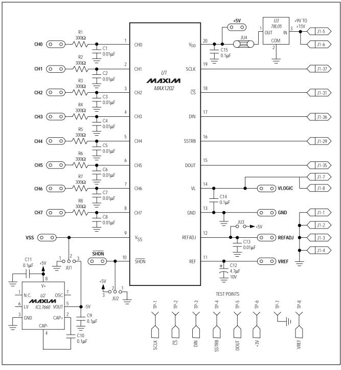
Figure 1. MAX1202 EV Kit Schematic
