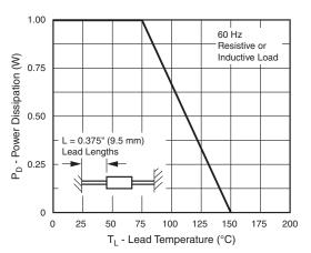
Fig. 4 - Pulse Derating Curve
