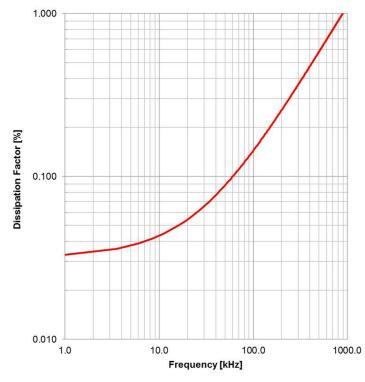
Test Equipment: E4991A or equivalent
