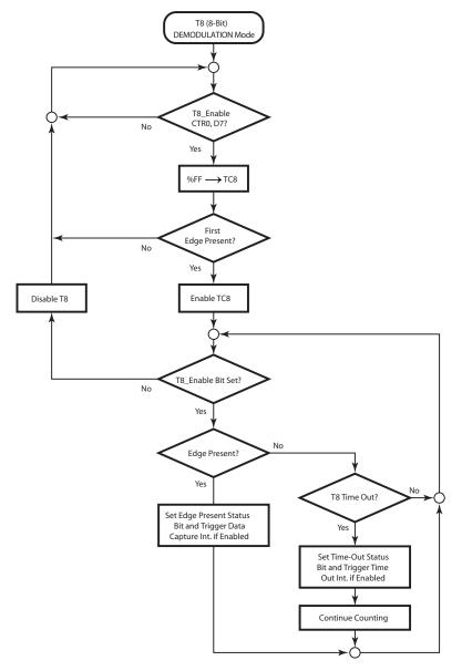
Figure 33. DEMODULATION Mode Flowchart
