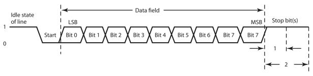
Figure 24. UART Asynchronous Data Format with Parity
