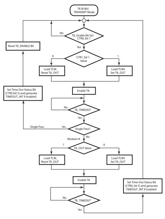
Figure 28. TRANSMIT Mode Flowchart
