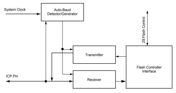
Figure 16. In-Circuit Programmer Block Diagram
