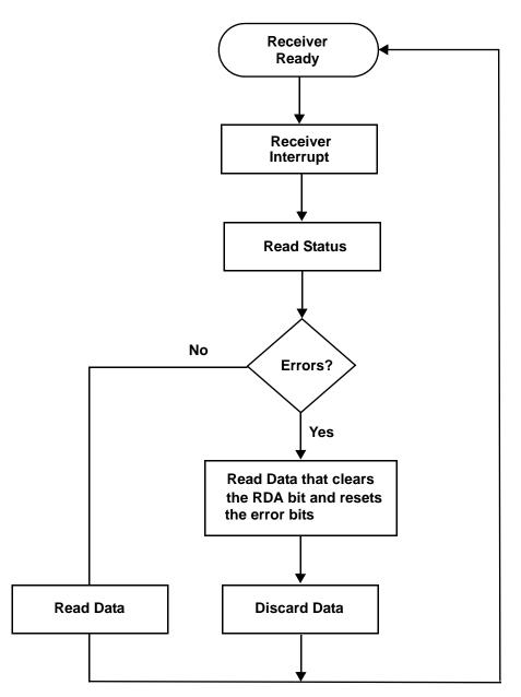
Figure 25. UART Receiver Interrupt Service Routine Flow
