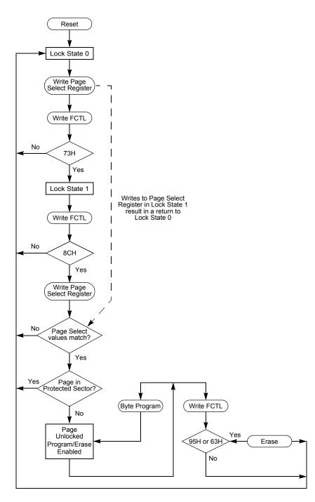
Figure 20. Flash Controller Operation Flow Chart
