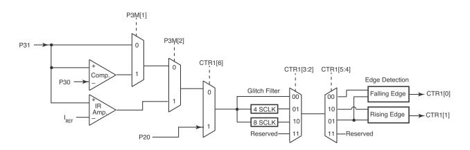
Figure 27. Counter/Timer Input Circuit
