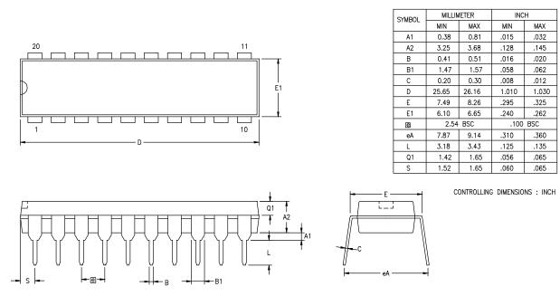
Figure 53 displays the 20-pin plastic dual inline package (PDIP) for the ZLF645 Series of Flash MCUs.
