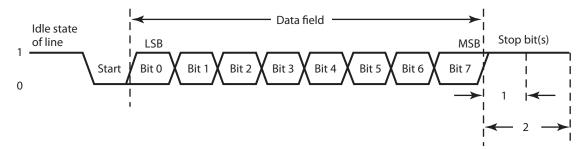
Figure 23. UART Asynchronous Data Format without Parity
