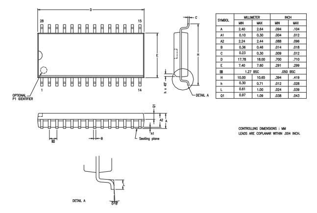
Figure 55. 28-Pin SOIC Package Diagram
