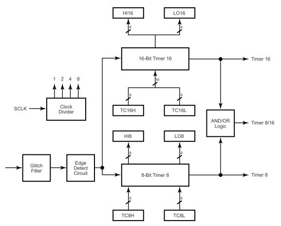
Figure 26. Counter/Timers Block Diagram
