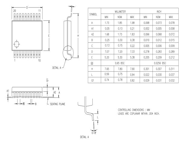
Figure 51. 20-Pin SSOP Package Diagram
