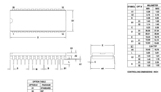
Note: Zllog supplies both options for production. Component layout PCB design should cover bigger option 01.
