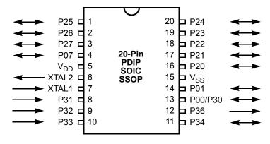
Figure 3. 20-Pin PDIP/SOIC/SSOP Pin Configuration
