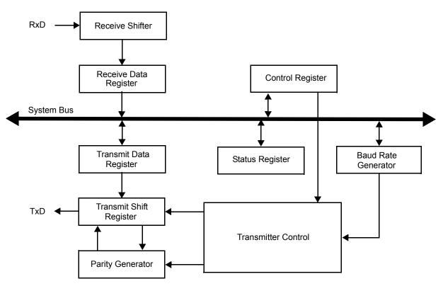
Figure 22. UART Block Diagram
