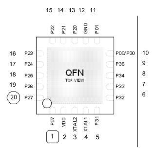
Figure 2. 20-Pin QFN Pin Configuration
