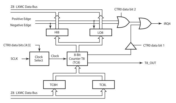
Figure 29. 8-Bit Counter/Timer Circuits
