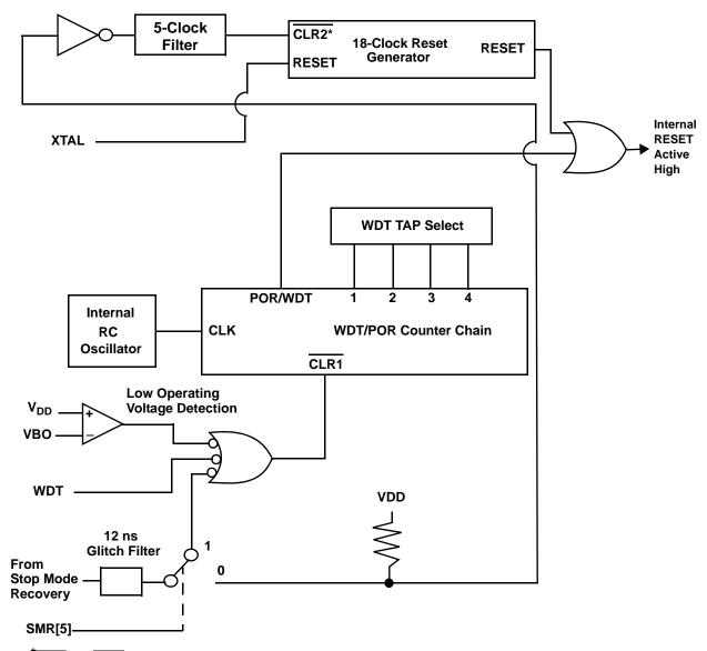
\* CLR1 and CLR2 enable the WDT/POR and 18 Clock Reset timers, respectively, on a Low-to-High input transition.
