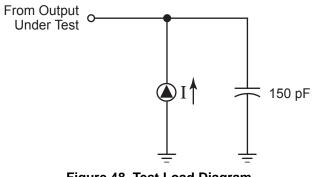
Figure 48. Test Load Diagram
