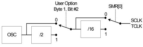
Figure 42. SCLK/TCLK Circuit
