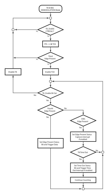
Figure 34. DEMODULATION Mode Flowchart with Bit 4 of CTR3 Set
