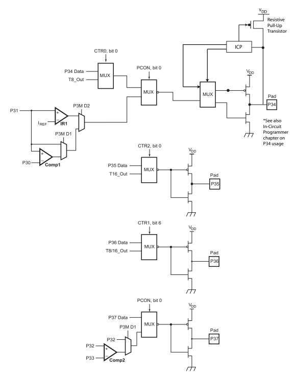
Figure 10. Port 3 Counter/Timer Output Configuration
