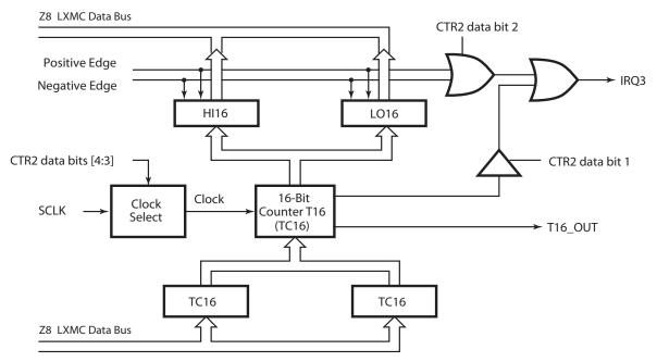
Figure 35. 16-Bit Counter/Timer Circuits
