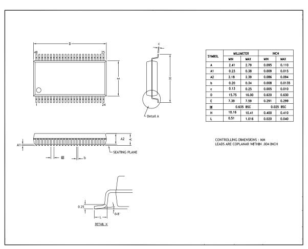
Figure 57 displays the 48-pin shrink small outline package (SSOP) for the ZLF645 Series of Flash MCUs.
