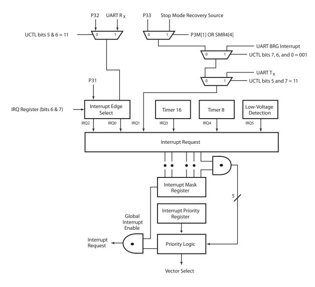
Figure 40. Interrupt Block Diagram
