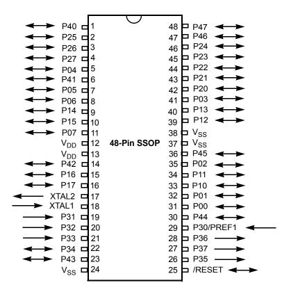
Figure 5. 48-Pin SSOP Pin Configuration
