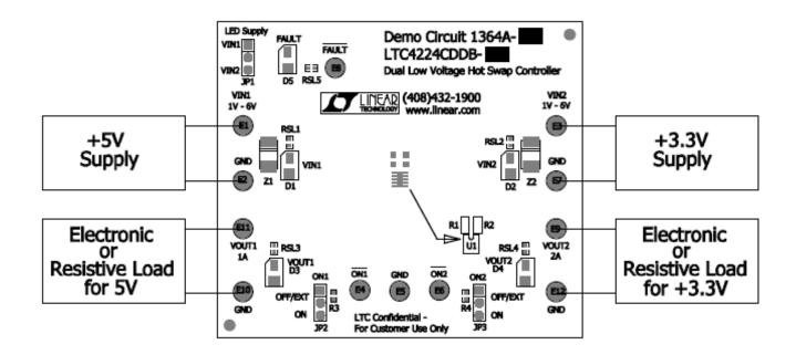
Figure 1. Proper Measurement Equipment Setup
