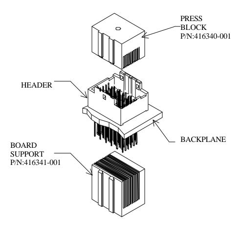
IF YOUR BACKPLANE IS GREATER THAN 4.30mm AND YOU ARE USING DASH NUMBERS X01, X02, AND X03 YOU WILL NOT NEED BOTTOM TOOLING AS THE TAIL WILL NOT EXTEND BELOW THE PC BOARD. IF YOUR BACKPLANE IS LESS THAN 4.30mm OR YOUR TAIL LENGTH IS GREATER THAN YOUR BACKPLANE YOU WILL NEED TO USE BOTTOM TOOLING.
