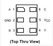
Figure 3. MicroPak (Top Through View)
