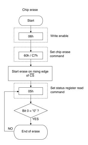
\* Automatically placed in write disabled state at the end of the erase
