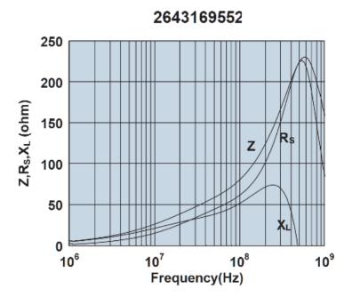
Impedance, reactance, and resistance vs. frequency.
