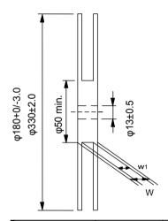
Fig.3 Taping Diagram
