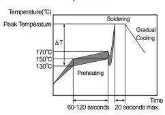
[Allowable Soldering Temperature and Time]
